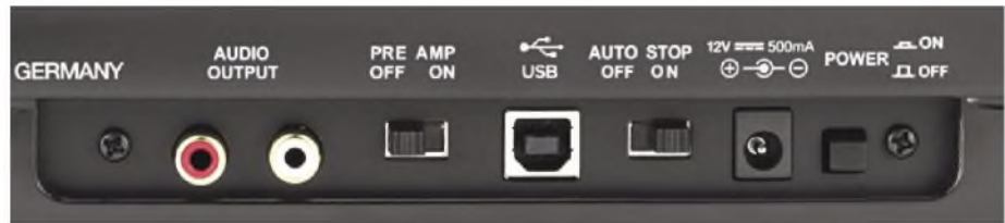
The rear panel with analogue phono output, preamp switch, USB B connector and 12V d.c. input from an external supply.
